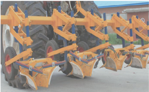
图1 马铃薯专用中耕培土犁 Fig. 1 Special ridging plough machine for potato
